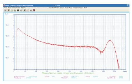
Figura. 5. The simulated spectrum of K-40 in sea water environment  $(A = 12500 \text{ Bq/m}^3)$ Living time: 3 days. Detector: NaI(Tl) (3" \* 3").
